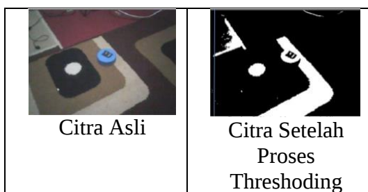
Gambar 9. Metode Threshold image processing Sumber: (Abimanyu K, Rohman S; 2019)
